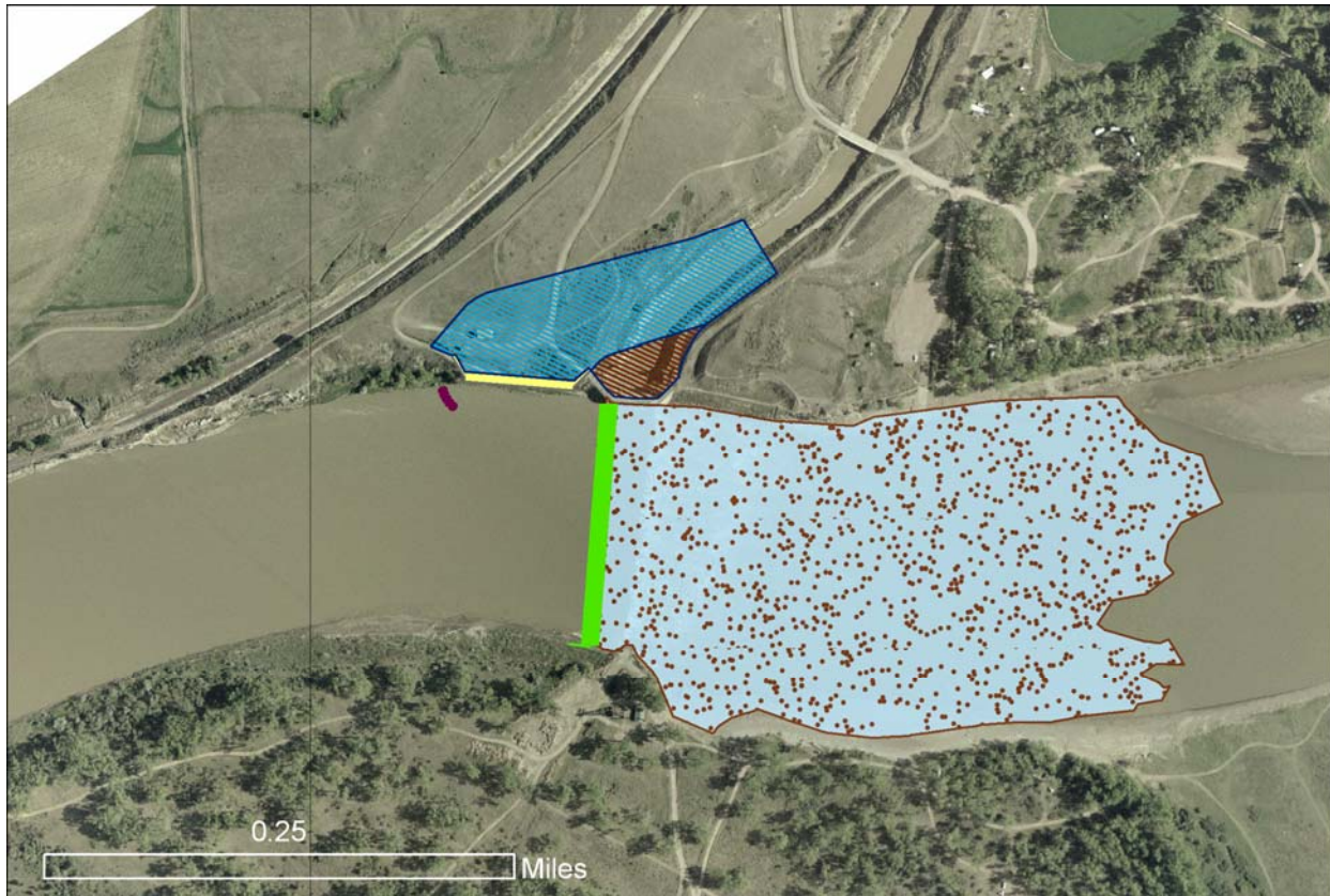
Figure 2.9 – Rock Ramp Alternative (concrete weir shown in green, rock ramp in light blue, canal extension in blue, new headworks in yellow, existing headworks in brown, and bollards in red).
